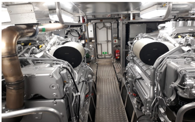
2 x 1660 HK dieselmotorer driver vannjet i 40 knop
